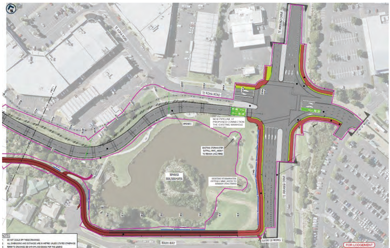
Figure 17: Existing and new stormwater infrastructure for EB4L
